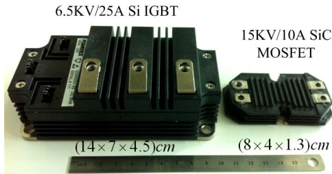
Fig. 3. Size comparison between Si IGBT and SiC MOSFET.
